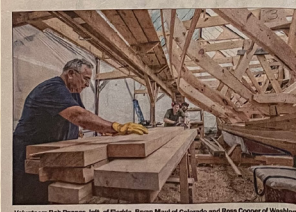
Volunteers Bob Pappas, left, of Florida, Bryan Mead of Colorado and Ross Cooper of Washington D.C., stack planks of rough-milled white oak after running it through a thickness planer.
